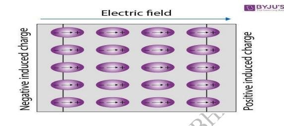
Let us consider a dielectric slab in an electric field which is acting in the direction shown in the figure. The arrangement of charges within the molecules of the dielectric in the electric field is as shown in the figure. The positive charges move in the direction of the field and the negative charges in the opposite direction. In other words, the electric dipoles align themselves with the direction of the field. In this state, the entire dielectric and its molecules are said to be polarized.
