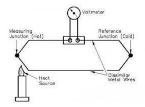
If the temperate at the junction end turn into equivalent, then the equivalent, as well as reverse electromagnetic force, produces in the circuit, and there is no flow of current through it. Similarly, the temperature at the junction end becomes imbalanced, then the potential variation induces in this circuit.
