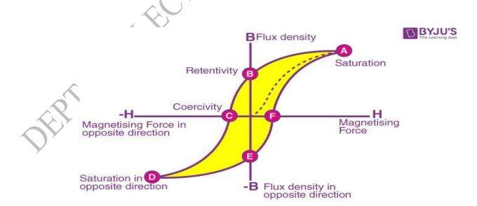
Looking at the graph, if B is measured for various values of H and if the results are plotted in graphic forms then the graph will show a hysteresis loop.
