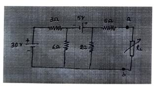
4. Draw Thevenin's equivalent circuit between terminal 'a' and 'b' of the above figure.
