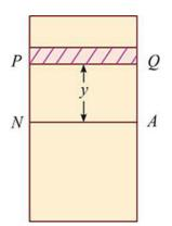
Now  $\sum y \cdot \delta a$  is the moment of the sectional area about the neutral axis, and since this moment is zero, the axis must pass through the centre of area.
