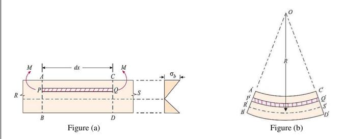
Now consider a layer PQ at a distance y from RS (the neutral axis of the beam). Let this layer be compressed to P'Q' after bending as shown in Figure (b).
