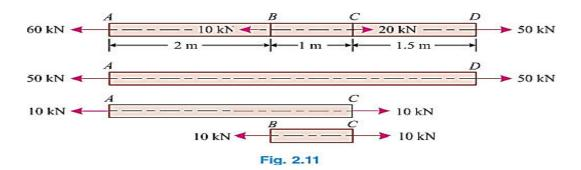
Now it will be seen that the bar AD is subjected a tensile force of 50 kN, part AC is subjected to a tensile force of 10 kN and the part BC is subjected to a tensile force of 10 kN as shown in Fig. 2.11 We know that deformation of the bar,
