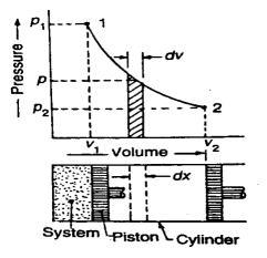
Let at any small section (shown shaded), the pressure (p) of the system is constant. If A is the cross-sectional area of the piston, then force on the piston (F = p A) causes the piston to move through a distance dx, Thus work done by the system,
