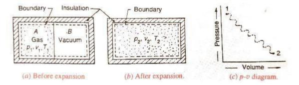
Consider two chambers A and B separated by a partition as shown in the figure (*a*). Let the chamber A contains a perfect gas having volume  $v_I$ , pressure  $p_I$ , and temperature  $T_I$ , and the chamber B is completely evacuated. These chambers are perfectly insulated so that no heat transfer takes place from or to its surroundings. Now, if the partition is removed, the gas will expand freely and occupy the whole space as shown in the figure (*b*).
