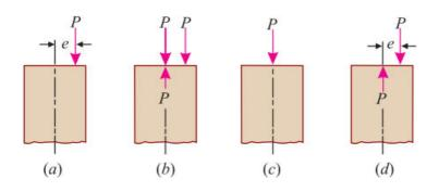
Consider a column subjected to an eccentric loading. The eccentric load may be easily analysed as shown in Figure above and as discussed below:
