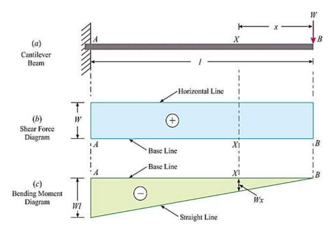
• Thus, from the equation of shear force, we see that the shear force is constant and is equal to W at all sections between B and A. And from the bending moment equation, we see that the bending moment is zero at B (where x = 0) and increases by a straight-line law to -Wl; at (where x = l).
