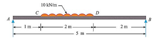
Solution. Given: Span (l) = 5 m; Uniformly distributed load (w) = 10 kN/m and length of the beam CD carrying load (a) = 2 m.
