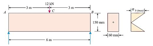
We know that maximum bending moment at the centre of a simply supported beam subjected to a central point load,
