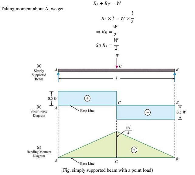
Thus, we see that the shear force at any section between A and C (i.e., up to the point just before the load W) is constant and is equal to the unbalanced vertical force, i.e., + 0.5 W. Shear force at any section between C and B (i.e., just after the load W) is also constant and is equal to the unbalanced vertical force, i.e., - 0.5 W as shown in Figure (b).
