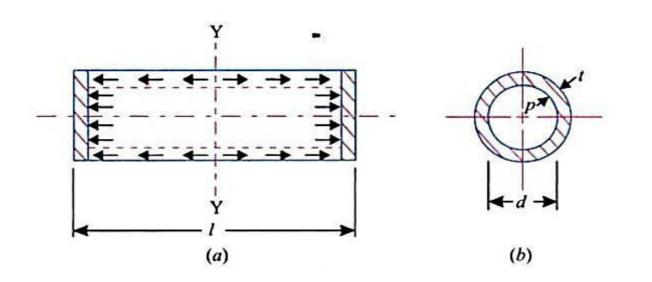
Bursting force = internal fluid pressure × area =  $P \times \frac{\pi}{4} \times d^2$
