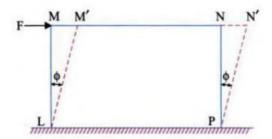
Consider a rectangular block LMNP fixed at one face and subjected to force 'F'. After application of force, it distorts through an angle 'φ' and occupies new position LM'N'P. the shear strain (*e<sub>s</sub>*) is given by,
