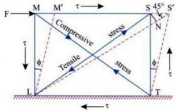
Consider a solid cube *LMST* subjected to a shearing force 'F'. Due to shearing load 'F' let the cube is distorted to *LM'S'T* and the diagonal *LS* to *LS'*. Let  $\tau$  be the shear stress produced in the faces *MS* and *LT* due to this shearing force.
