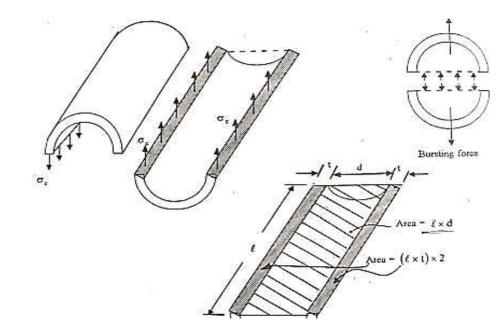
Let P = Internal fluid pressure inside the cylinder  $\sigma_c$  = Circumferential or Hoop stress d = Internal diameter of the cylinder t = Thickness of the cylinder
