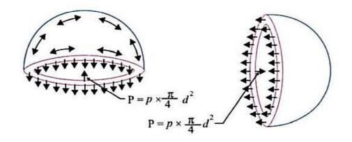
Bursting force = internal fluid pressure × area  $= P \times \frac{\pi}{4} \times d^{2}$ Resisting force = circumferential stress × area on which it acts  $= \sigma_{c} \times \pi \times dt$ For equilibrium Resisting force = bursting force  $\Rightarrow \sigma \times \pi \times dt = P \times \frac{\pi}{4} \times d^{2}$   $\Rightarrow \sigma_{c} = \frac{Pd}{4t}$
