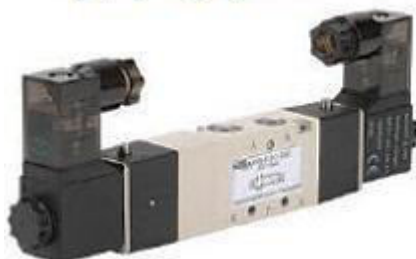
4-way (5-port), 3-position closed center, double-piloted solenoid, spring centering
