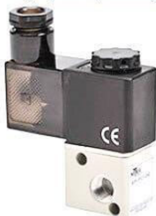
3-way, 2-position, normally closed direct-acting solenoid valve, spring return
