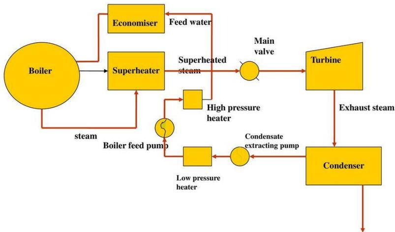
After expanding in the turbine, the steam is again circulated through here heater to gain the original dryness. After that it is finally enter into the condenser for condensation.
