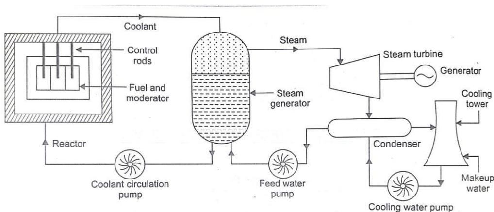
(i) **Reactor:** Nuclear fission reaction takes place inside a reactor. The heat generated due to chemical reaction is carried away by a coolant to a heat exchanger or boiler where steam is raised. Reactor is built with a core having fuel pellets and coolant surrounds the fuel pellets. Control rods are used to regulate the speed of chain reaction. A number safety mechanism is built in to protect the core from abnormal operation.
