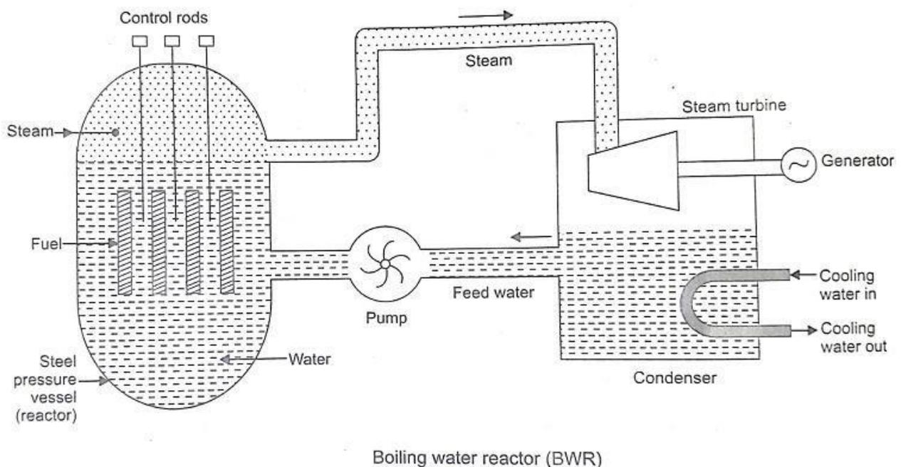
Feed water enters at the bottom and gets evaporated into steam due to heat of fission reaction. This steam leaves the reactor at the top and enters the steam turbine. After expansion of steam in the steam turbine, it gets condensed in a water-cooled condenser and fed back to the heat exchanger as feed water. Due to radioactive contamination around the reactor core, radiological protection is provided to the steam turbine.
