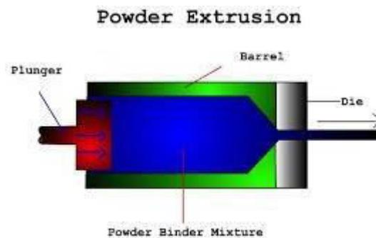
In this process the powder is canned and placed in some kind of metal container. The sealed container is heated and then extruded. After extruding, the container material is removed either mechanically or chemically. This technique is extremely used for high densities of production.
