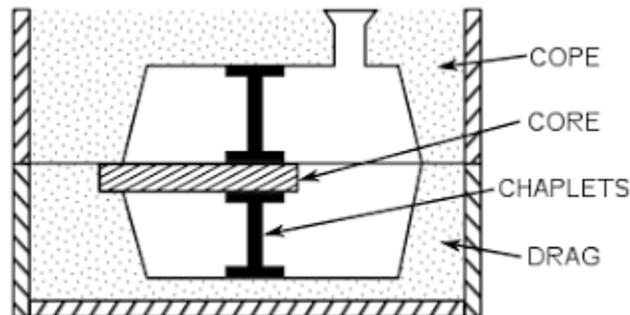
A core may be defined as a sand shape or from which makes the cavity of a casting for which no provision has been made in the pattern for moulding.
