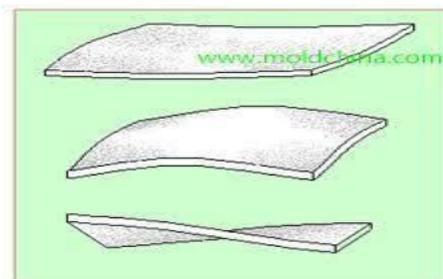
Casting warp or deform because of stress set up in them internally ,due to different solidification rate experienced by different sections of large, long and wide flat castings.
