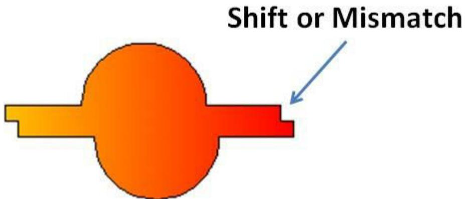
It produces a casting which does not match at the parting line.
