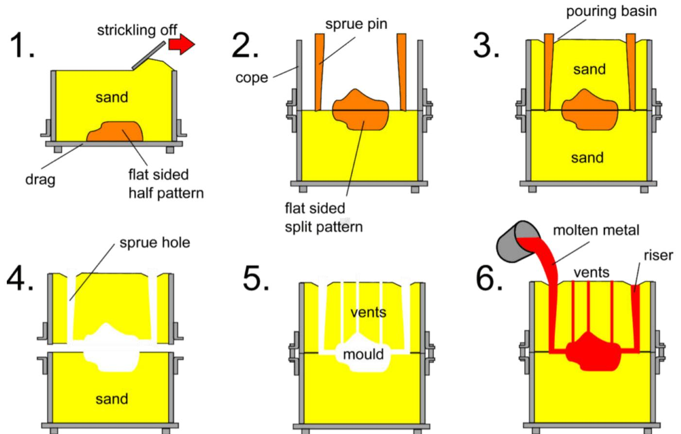
1. **Selection of sand**:-Select the sand for preparation of mould box. The sand should have good mechanical as well as thermal properties like binding property and permeability.
