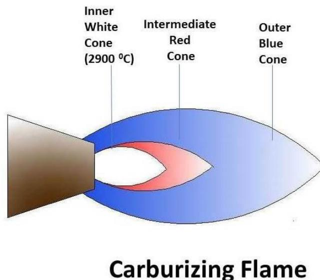
It is otherwise called as carburising flame. If the volume of oxygen supplies to the neutral flame is reduced and acetylene is increased the resulting flame will be reducing flame. A reducing flame is recognised by acetylene feather which exist between inner cone and outer envelope. The outer envelope is longer then the neutral flame and is much brighter in colour. Reducing flame has a temperature of 3038<sup>0</sup>C. A reducing flame is used in welding of lead, low alloy steel etc.
