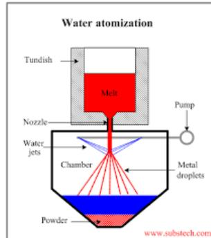
In atomisation process, the metal is forced through a small orifice called nozzle and is disintegrated by a stream of compressed air or water jet and then cooled into fine powders .since the particles are very small like atoms, this process is called atomisation. Oxidation of the metal powder can be prevented by maintaining inert atmosphere. This process generally used for metals having low melting point.
