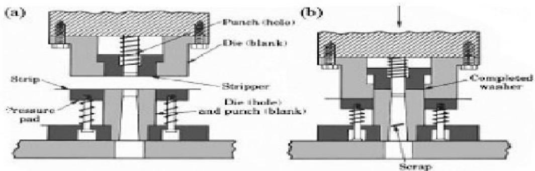
Fig 16.11 Schematic illustrations: (a) before and (b) after blanking a common washer in a compound die. note the separate movements of the die (or blanking) and the punch
