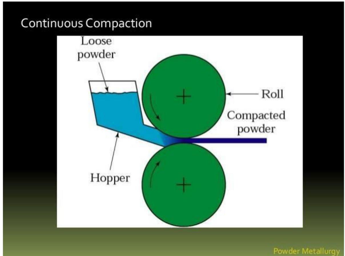
In powder rolling, the rolls are set side by side so that the strip emerges vertically downwards. The continuous feeding of the powder produces the strip of infinite length. Then the strip is sintered for a very short time.
