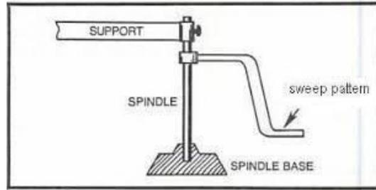
To produce complex 3d objects using 2d plane pattern we use this pattern.
