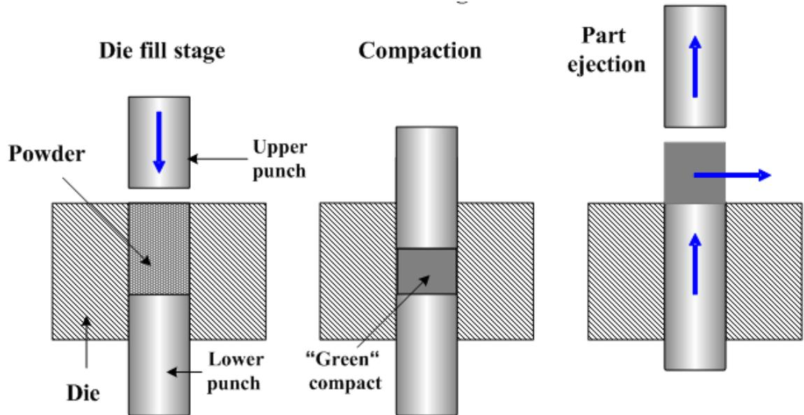
Dies are usually made of ground , hardened steels .The die consists of two parts lower punch and upper punch. The metal powder is introduced into the cavity of the die. Required pressure is given by movement of upper and lower punches towards each other, after the green compact is ejected from the lower punch. This pressure commonly employed ranges from 19-50 tons/sq. inch. It may be obtained by hydraulic or mechanical.
