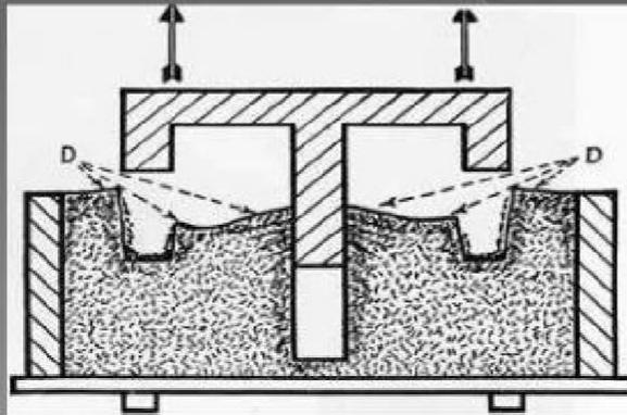
When the pattern is shaken for easy withdrawal the mould cavity gets slightly larger in dimension. This also causes the casting size to increase for compensating this factor the pattern should initially be made slightly smaller than the desired size.
