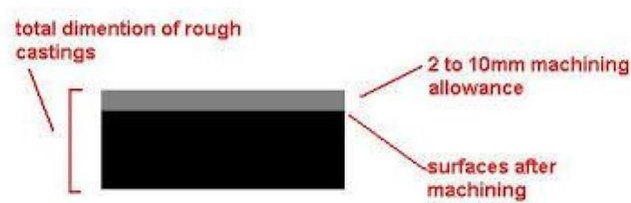
Machining allowances is the finishing allowances which is given in the pattern to get better surface finish. It depends on the size, shape and volume of casting, configuration of casting, characteristics of metal etc.
