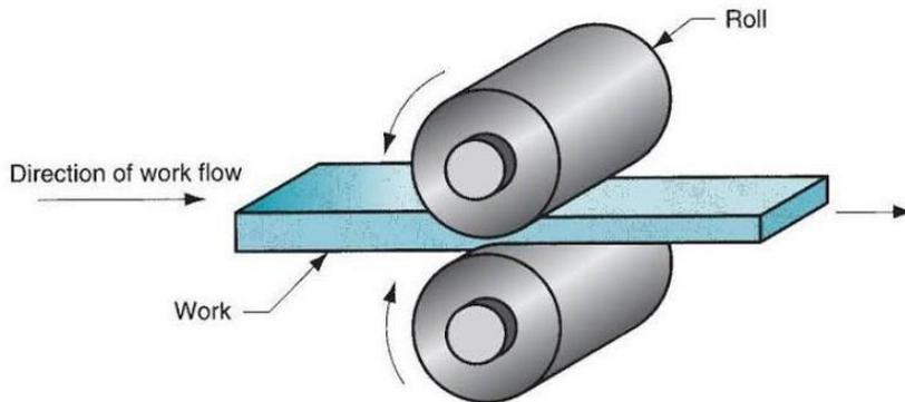
In metal working, rolling is a metal forming process in which a metal stock passed through one or more pair of rolls to reduce the thickness and to make the thickness uniform.
