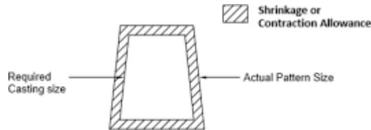
**Figure. Shrinkage or contraction Allowance**
