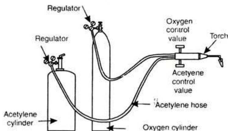
**Fig. 7.3. Oxy-acetylene welding equipment.**
