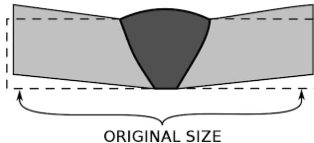
Distortion is the change in shape and difference between the position of the two work pieces before welding and after welding.
