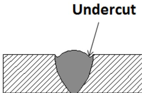
If the groove gets formed in the parent metal along the side of the weld bead that is called under cutting.
