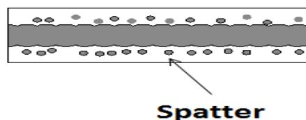
Spatter refers to small particles of metals, which are scattered around the weld along its length.
