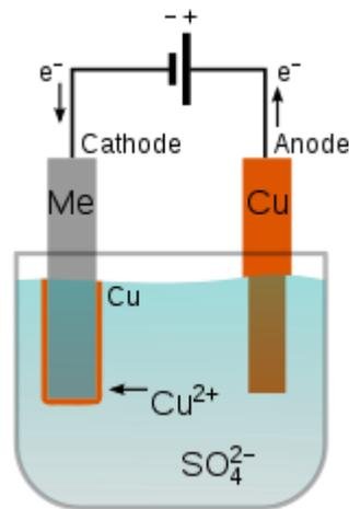
The principle involved in this method is similar to that of electrolysis, during which a powdery deposit is obtained in the cathode. The deposit powder is scrapped, washed, dried and then pulverised further to get fine powder of desired size.
