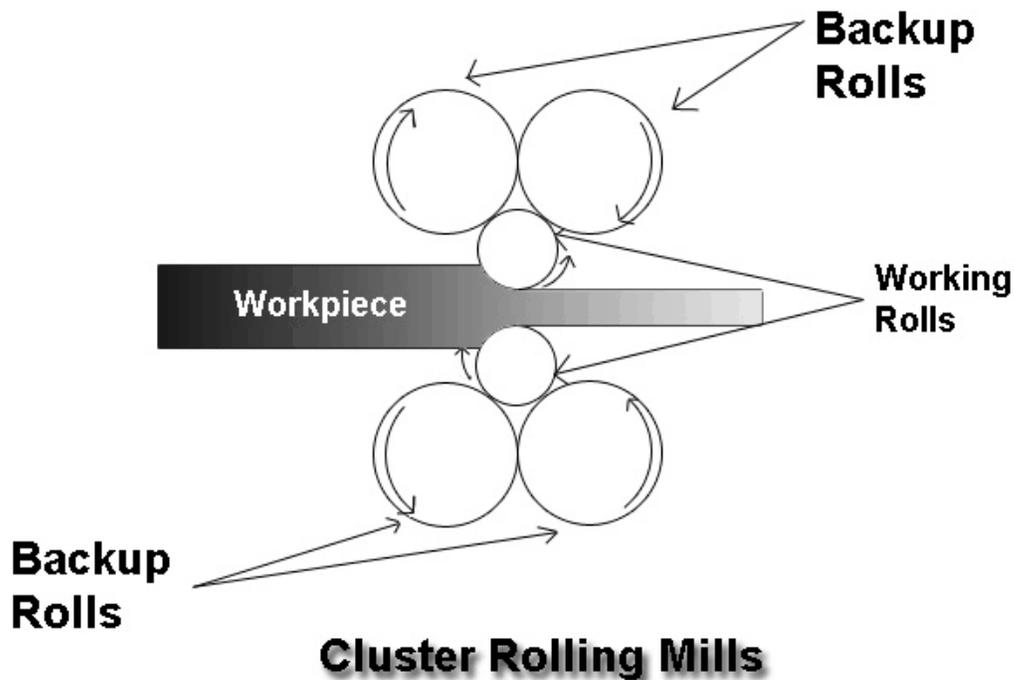
It is a special type of four high rolling mill in which each of the two working rolls is backed up by two or more of the larger backup rolls for rolling hard in material. It may be necessary to employ work rolls of a very small diameter but of considerable length.
