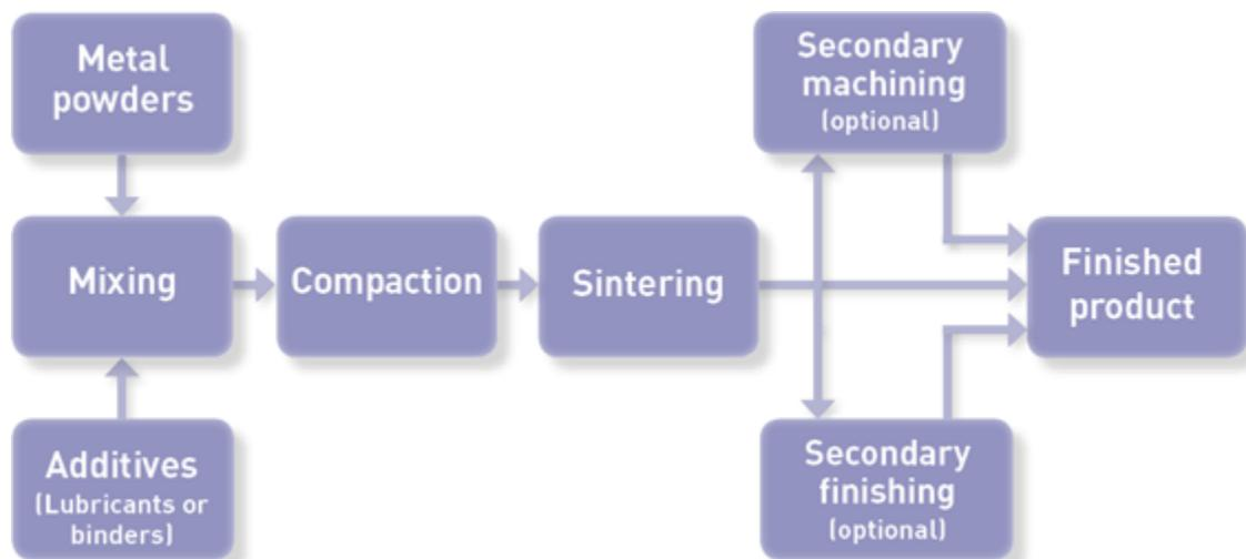
The powder metallurgy process consists of four basic steps :-
