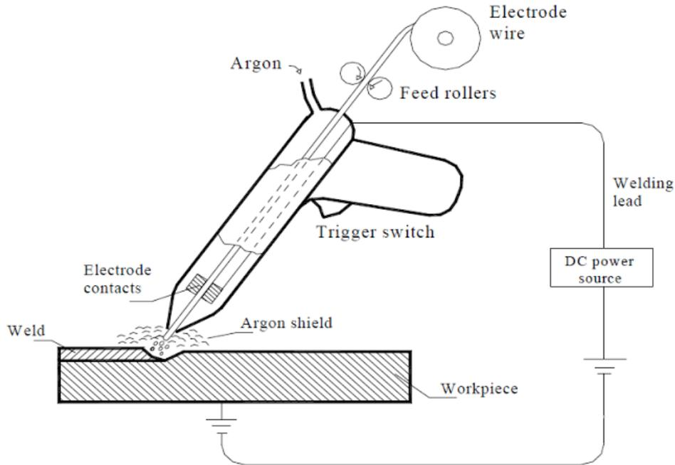
The following components are necessary to perform metal inert gas welding.
