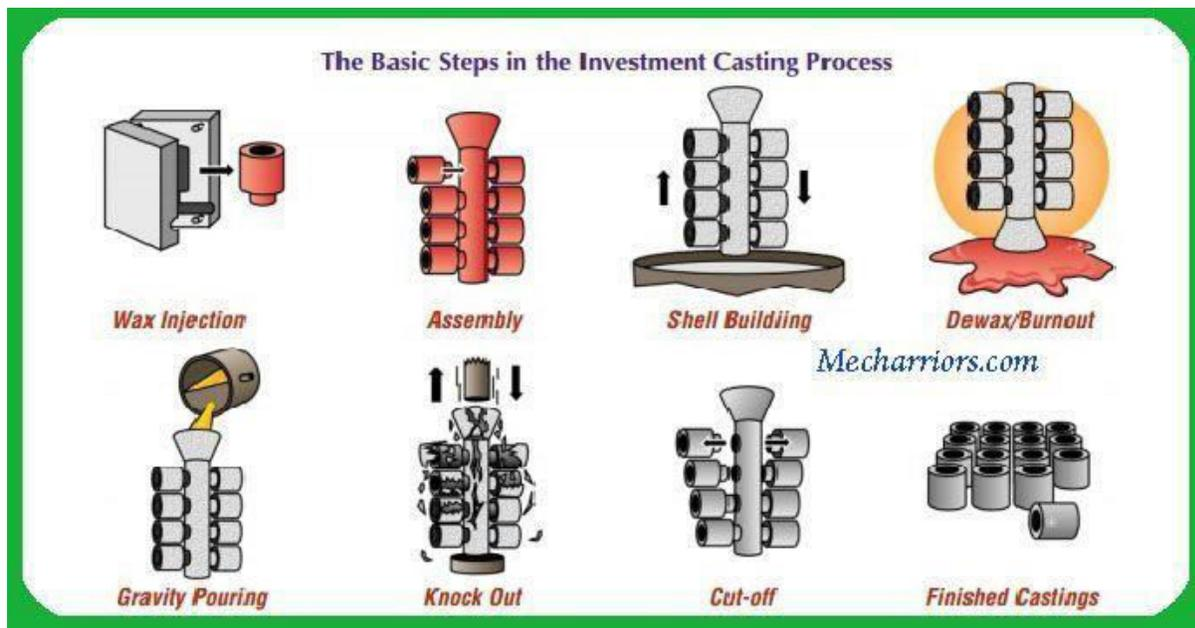
Investment casting is one of the oldest manufacturing process, dating back 1000 of years ,in this process molten metal is poured into an expandable ceramic mould.
