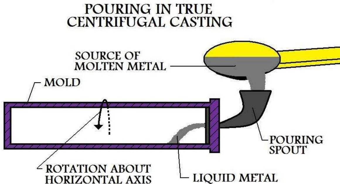
True centrifugal casting are of straight uniform inner diameter and are produced by spinning the mould about its own axis, either vertically or horizontally.
