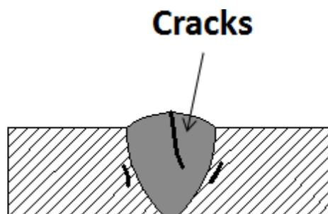
Cracks may occur in various locations and directions such as in the weld , root etc.
