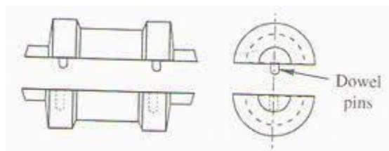
This is used when casting components having complex design. It is split along the parting surface.
