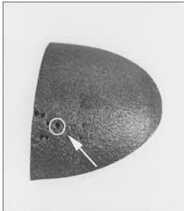
Pin holes are numerous very small holes revealed on the surface of a casting after the surface has been cleaned by shot blasting.
