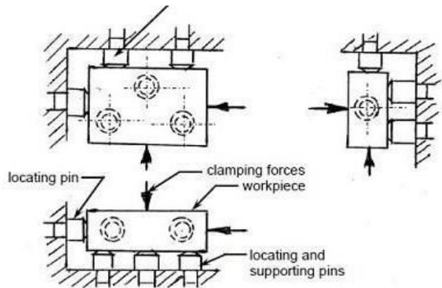
*Arresting all degrees of freedom of a blank in a fixture.*
