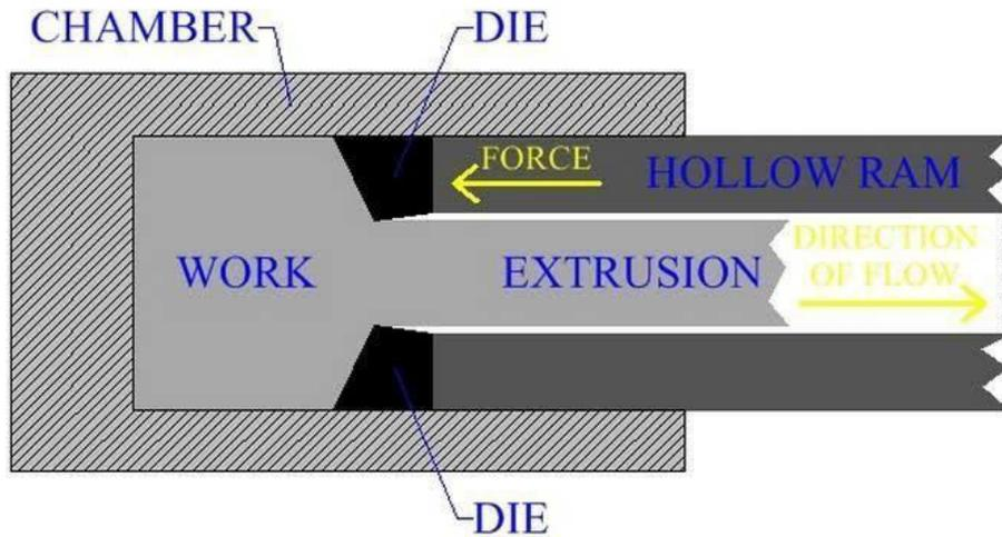
This process consists of a container, a ram and a die. In this process hot billet remains stationary, while die is pushed into the billet by a hollow ram through which extrusion takes place. Indirect extrusion does not require as much force as compared to direct extrusion because no force is required to move the hot billet inside the chamber wall. The length of the product in indirect extrusion is the size of the ram. Indirect extrusion method is also a hot working process.
