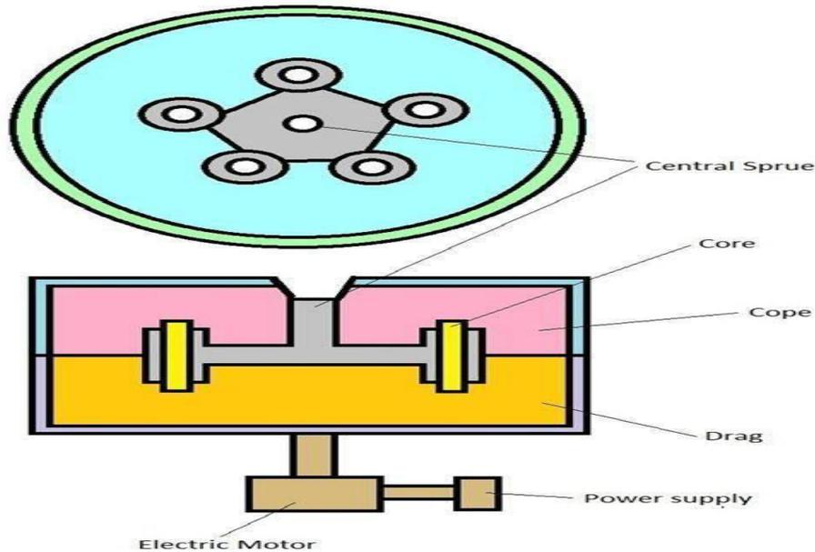
Parts not symmetrical about any axis of rotation may be cast in a group of mould arranged in a circle to balance each other.
