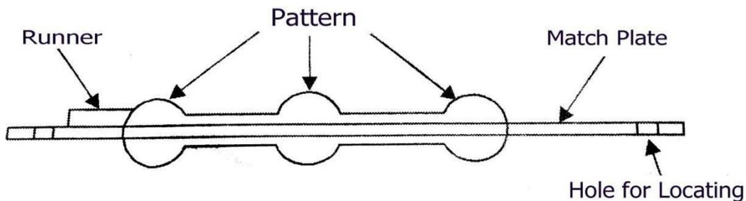
To produce small size components having more complex shape in mass production we can use this pattern.
