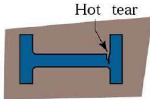
They are internal or external cracks having ragged edges occurring immediately after solidification.
