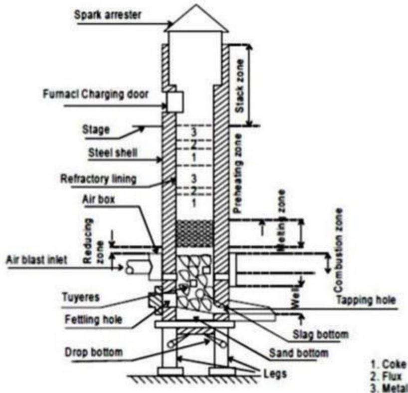
A cupola is a cylindrical shell constructed (welded or riveted) from boiler plate (6 to 10 mm) is open at both its top and bottom and is lined with firebrick and clay.
