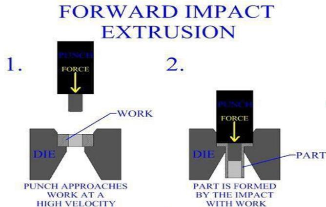
It is a cold working extrusion process. This method is same as hot extrusion method except that in impact extrusion the metals working without application of heat. The metals used in this process most have high degrees of ductility. The purpose of impact extrusion is mostly that producing a finished product. In this process a punch is used to force the metal work piece into the die cavity to take the shape of the cavity. Collapsible tubes of leads, tin and aluminium are produced by this method.
