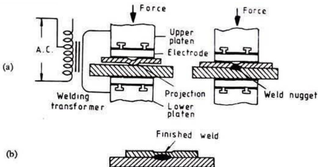
Fig. 2-20 Projection welding (a) Setup (b) Finished weld.
