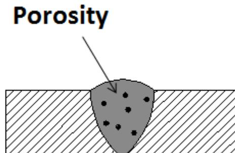
Porosity is the condition in which the gas or small bubbles gets trapped in the welded zone. Blow holes are the large gas cavities or bubbles create in the welded zone.
