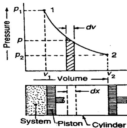
Let at any small section (shown shaded), the pressure ( $p$ ) of the system is constant. If  $A$  is the cross-sectional area of the piston, then force on the piston ( $F = p A$ ) causes the piston to move through a distance  $dx$ , Thus work done by the system,
