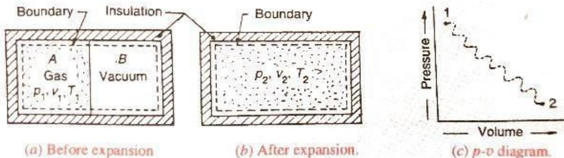
Consider two chambers *A* and *B* separated by a partition as shown in the figure (a). Let the chamber *A* contains a perfect gas having volume  $v_1$ , pressure  $p_1$ , and temperature  $T_1$ , and the chamber *B* is completely evacuated. These chambers are perfectly insulated so that no heat transfer takes place from or to its surroundings. Now, if the partition is removed, the gas will expand freely and occupy the whole space as shown in the figure (b).
