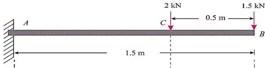
**Solution.** Given: Span ( $l$ ) = 1.5 m; Point load at B ( $W_1$ ) = 1.5 kN and point load at C ( $W_2$ ) = 2 kN.
