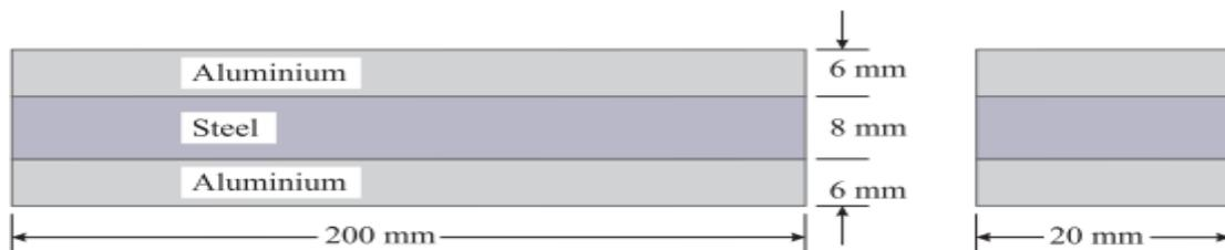
All the three bars are fastened together at room temperature. Find the stresses in each bar, Where the temperature of the whole assembly is raised through  $50^\circ\text{C}$ . Assume:
