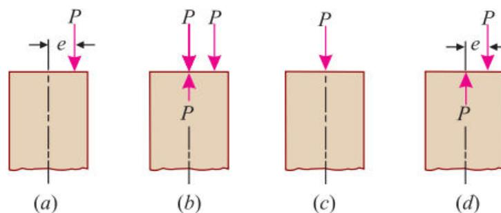
Consider a column subjected to an eccentric loading. The eccentric load may be easily analysed as shown in Figure above and as discussed below:
