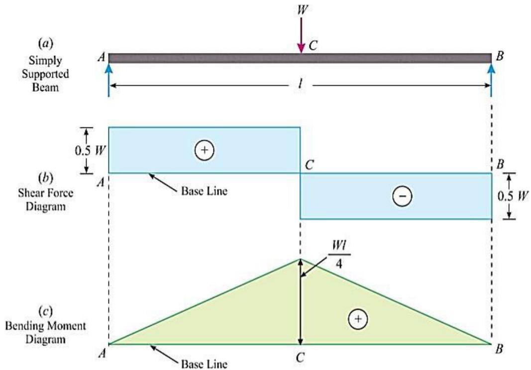
(Fig. simply supported beam with a point load)
