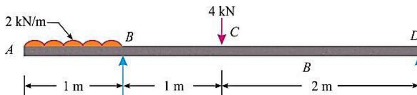
Solution. Given: Span ( $l$ ) = 4 m; Uniformly distributed load over AB ( $w$ ) = 2 kN/m and point load at C ( $W$ ) = 4 kN.
