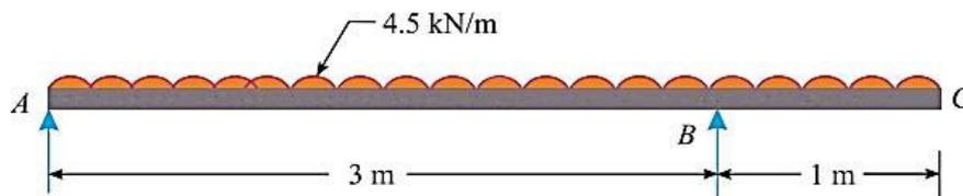
Solution. Given: Span ( $l$ ) = 4 m; Uniformly distributed load ( $w$ ) = 4.5 kN/m and overhanging length ( $c$ )=1m.
