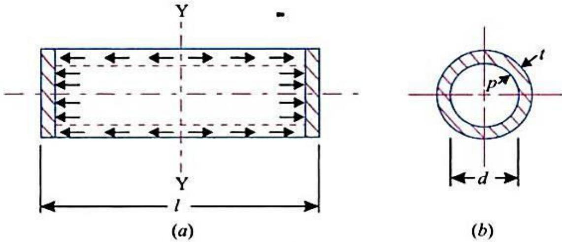
Bursting force = internal fluid pressure  $\times$  area
