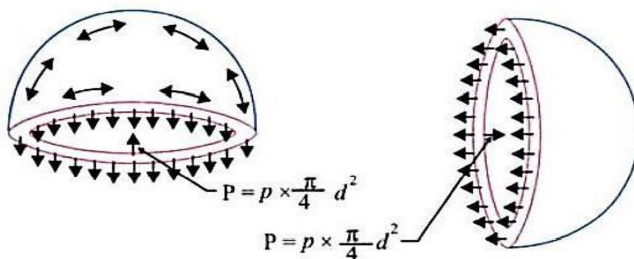
Bursting force = internal fluid pressure  $\times$  area
