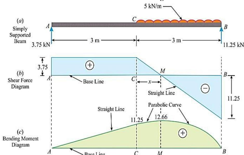
**Example – 5:** A simply supported beam 5 m long is loaded with a uniformly distributed load of 10 kN/m over a length of 2 m as shown in Figure. Draw shear force and bending moment diagrams for the beam indicating the value of maximum bending moment.
