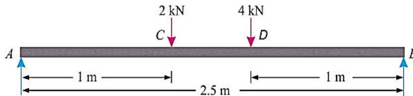
**Solution.** Given: Span ( $l$ ) = 2.5 m; Point load at C ( $W_1$ ) = 2 kN and point load at B ( $W_2$ ) = 4 kN.
