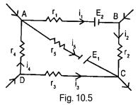
Figure 10.5 shows a closed electric circuit ABCD containing resistance  $r_1, r_2, r_3, r_4$  and  $r_5$  in the parts AB, BC, CD, DA and AC respectively. Also let  $i_1, i_2, i_3, i_4$ ,  $i_5$  be the respective currents flowing in these parts in the directions shown by arrow heads. Two sources of emf<sup>s</sup>  $E_1$ ,  $E_2$  are also connected in the mesh.
