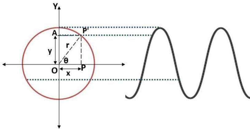
The projection of the motion of particle makes a simple harmonic motion along the diameter of the circle of reference. *Figure 6.2*
