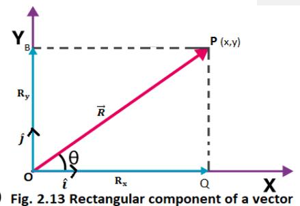
Fig. 2.13 Rectangular component of a vector
